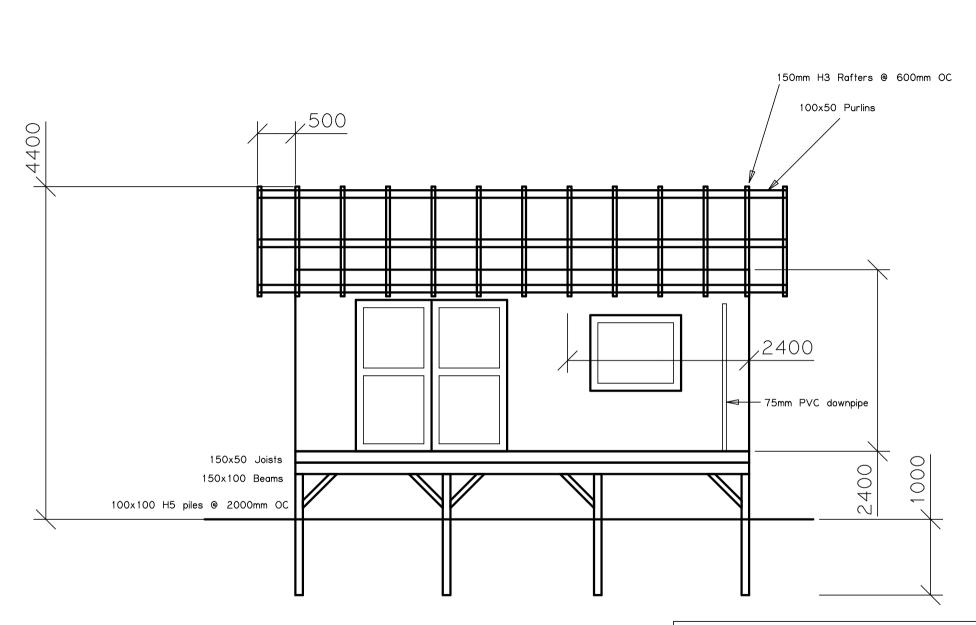
All wall framing 100x50 H3 PG VSG8 @ 400mm OC Window/Door headers 2x150x50 with plywood joiner Doors to comply to NZS4223 Pt 3
